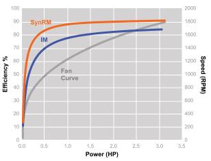
Even compared to premium efficient induction (IE3) motors up to 15 kW run with VFD's, PM-SynRM's have roughly a 3-5% efficiency improvement at 25-100% load. This gives a very quick payback in energy savings.
